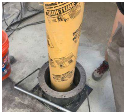
Fig. 1. Minimum density samples are prepared by removing a soil filled tube thus releasing the sample into the mold at an approximate minimum density.
