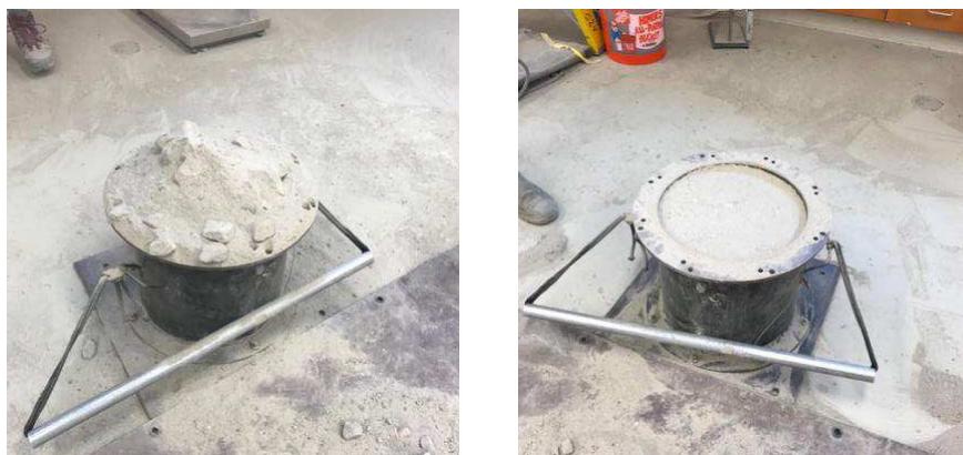
Fig. 2. Minimum Density 60% Fouling and 40% Railroad Ballast cylinder samples. On the left is the sample after being placed into the cylinder mold, and the right is after the excess is removed to the approximate correct volume.
