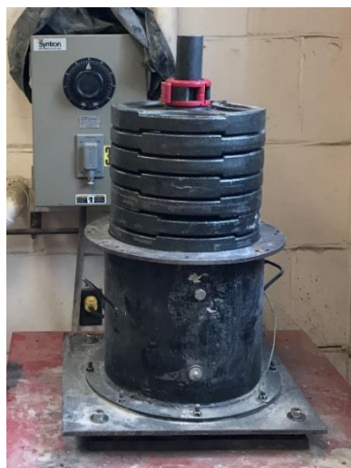
Fig. 2. Maximum density set up with cylinder, surcharge weights, and shaker table.
